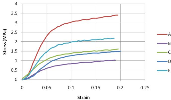
Figure 3. Quasi-Static Stress-Strain Response of Polyurethane ( $0.03 \text{ s}^{-1}$ ).
