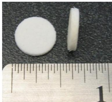
Figure 4. High Strain Rate Test Specimen Used in a Split Hopkinson Pressure Bar
