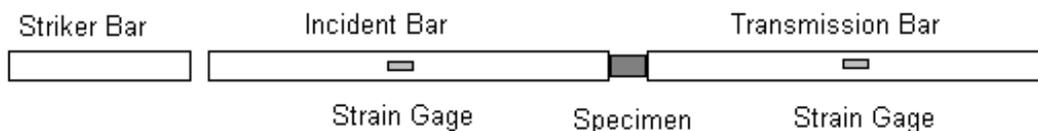
Figure 1. Diagram of a Split Hopkinson Pressure-Bar Apparatus.
