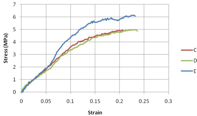
Figure 5. Impact Stress-Strain Response ( $2780 \text{ s}^{-1}$ ) for Polyurethanes of similar DS.
