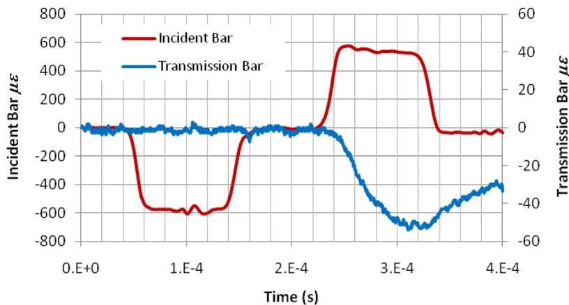
Figure 2. Representative pressure bar strain output for polyurethane.
