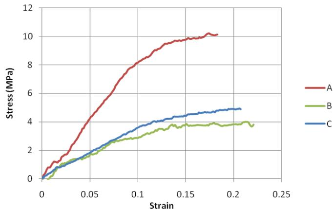
Figure 6. Impact Stress-Strain Response ( $2780 \text{ s}^{-1}$ ) for Polyurethane of similar COR.
