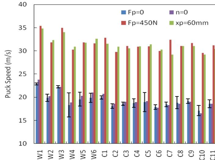
Figure 2: Stick performance for the cases of: no stick loading ( $F_p=0$ ), constant swing speed ( $n=0$ ), constant stick force ( $F_p=450\text{N}$ ), and constant stick displacement ( $x_p=60\text{ mm}$ ).
