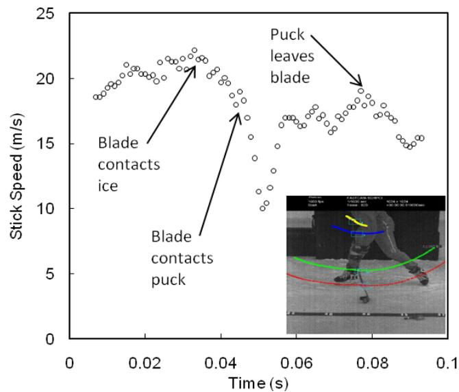
Figure 1. Stick speed measured 10 cm from the blade (red markers) during a slap shot.
