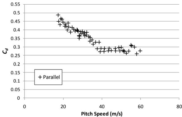
Figure 7 – Drag coefficient of MLB baseballs in the parallel orientation.
