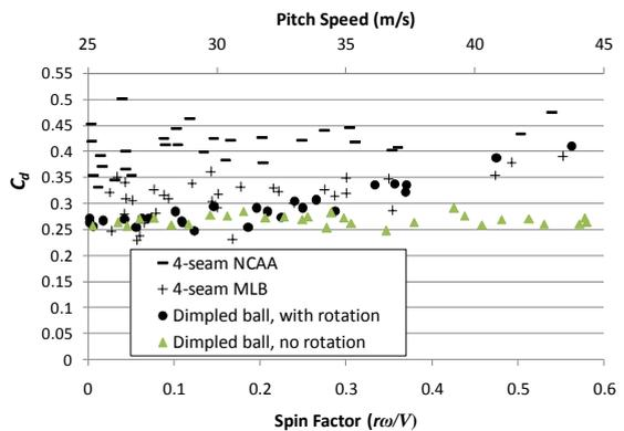
Figure 8. Drag coefficient of baseballs rotating in the normal and parallel orientations compared to a dimpled baseball.
