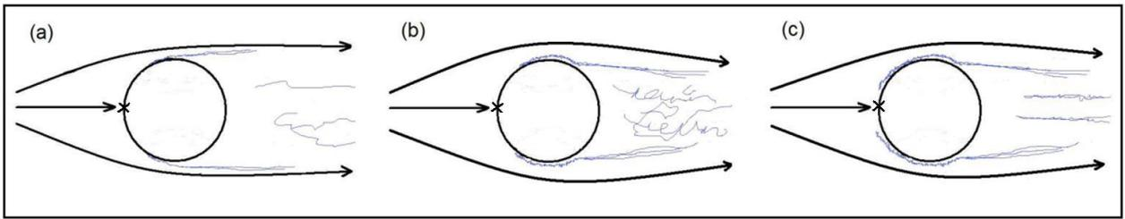
Figure 1 - Flow over a smooth cylinder: (a)  $R_e < 3 \times 10^5$ , flow stays laminar in the boundary layer until  $80^\circ$  where it separates; (b)  $3 \times 10^5 < R_e < 3 \times 10^6$ , flow separates at  $80^\circ$  becomes turbulent and reconnects before separating again at  $120^\circ$ ; (c)  $3 \times 10^6 < R_e$ , flow is turbulent in the boundary layer on the front and stays turbulent until separating at  $120^\circ$ . The stagnation point is identified by “X” in each figure.
