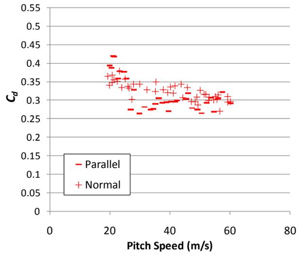
Figure 6. The drag coefficient of cricket balls in the normal and parallel orientations.
