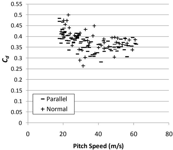
Figure 5. The drag coefficient of NCAA baseballs in the normal and parallel orientations.
