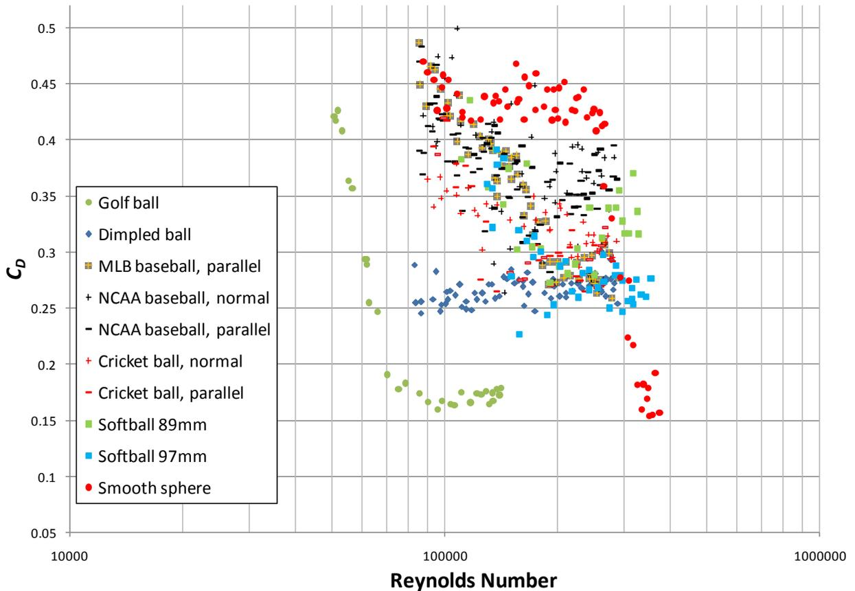
Figure 4. Coefficient of drag for all test balls.
