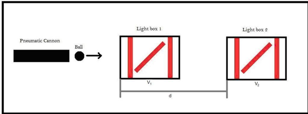
Figure 2. Diagram showing arrangement of pitching device and light boxes used to measure ball speed and location.
