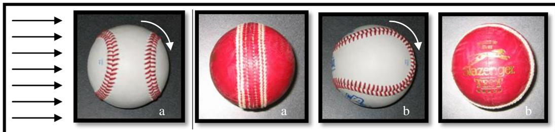
Figure 3. Diagram showing the normal (a) and parallel (b) orientations. Black arrows indicate the airflow direction, white arrows indicate the ball rotation axis.
