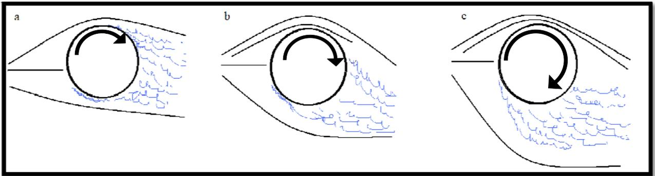
Figure 1 - Flow from left to right over a rotating smooth cylinder. Angular velocity, in the clockwise direction, increases in speed from a) to b) to c).
