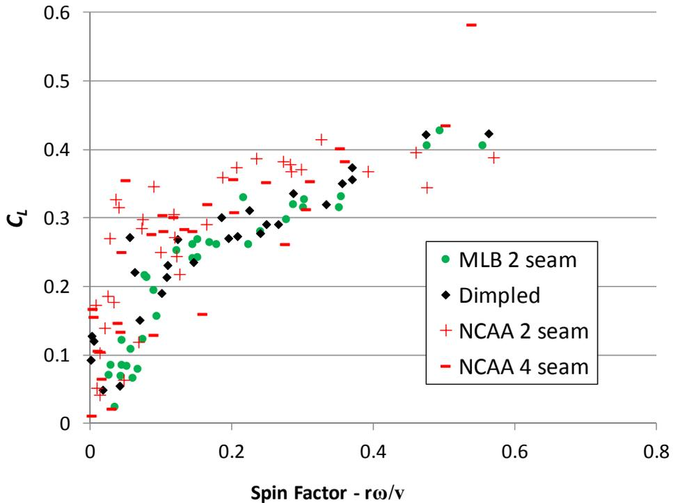
Figure 4. Coefficient of lift for all test balls.
