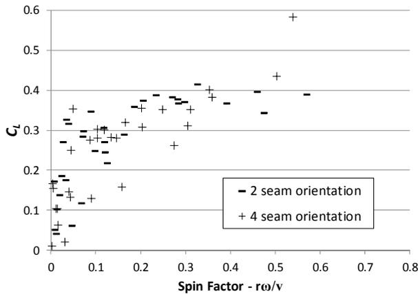
Figure 5. The lift coefficient of the collegiate baseball in the normal and parallel orientations.
