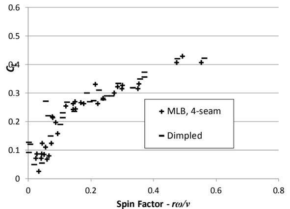
Figure 6. The lift coefficient of MLB in 4 seam orientation and the dimpled ball.
