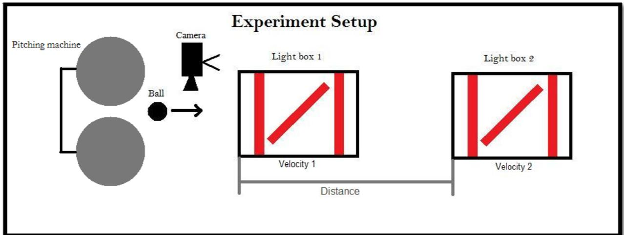
Figure 2. Diagram showing arrangement of pitching device and light boxes used to measure ball speed, rotation, and location.
