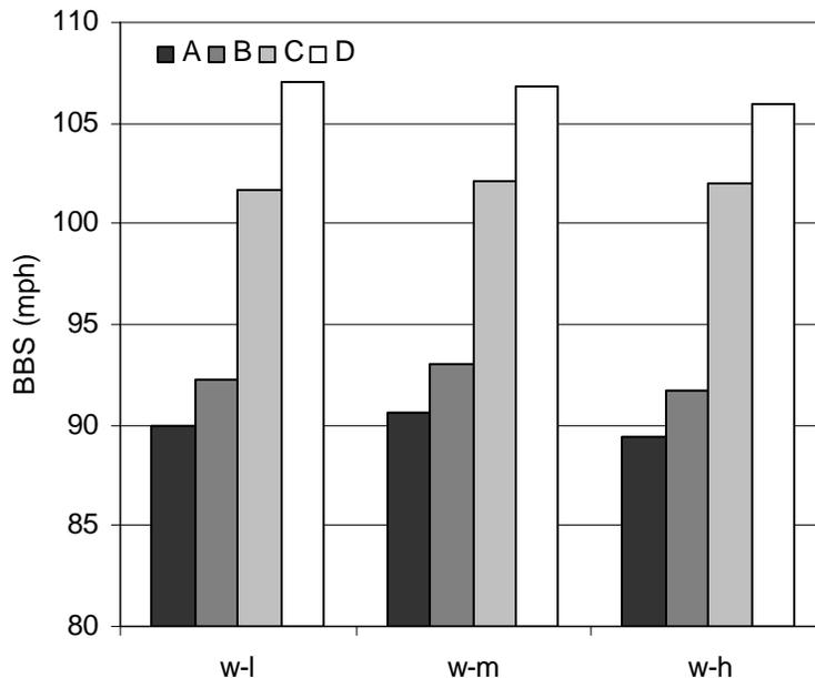
Fig. 1. BBS of four bats of differing performance using test balls of varying weight.
