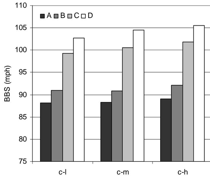
Fig. 2. BBS of four bats of differing performance using test balls of varying compression.
