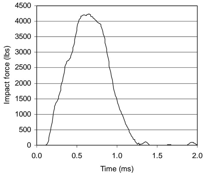
Fig. 5. Impact force of a softball against a rigid cylinder at 95 mph.
