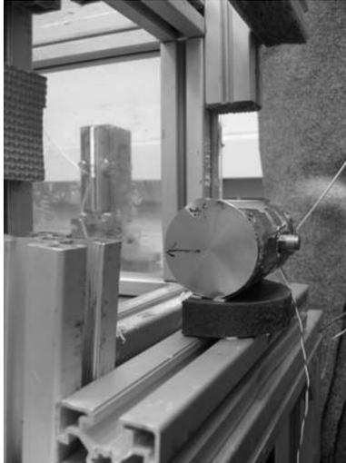
Fig. 6. Picture of recoiling solid cylinder with accelerometer on the back side.
