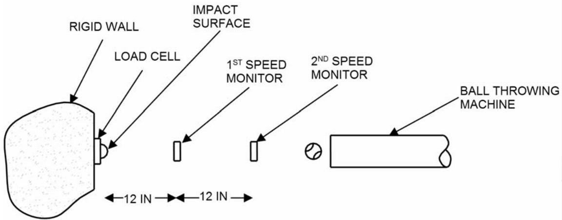
Fig. 4. A schematic depiction showing how dynamic stiffness is measured.
