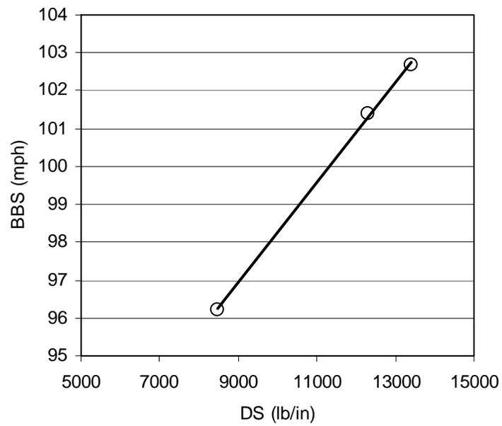
Fig. 7. A comparison of BBS and dynamic stiffness for a bat tested with balls of similar COR and compression.
