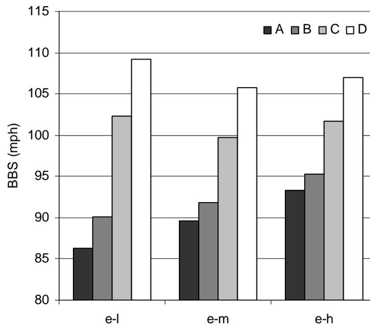
Fig. 3. BBS of four bats of differing performance using test balls of varying COR.
